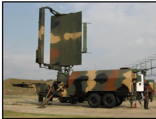
Figure 6-9 Tin Shield TA Radar Mounted On Mobile Chassis
