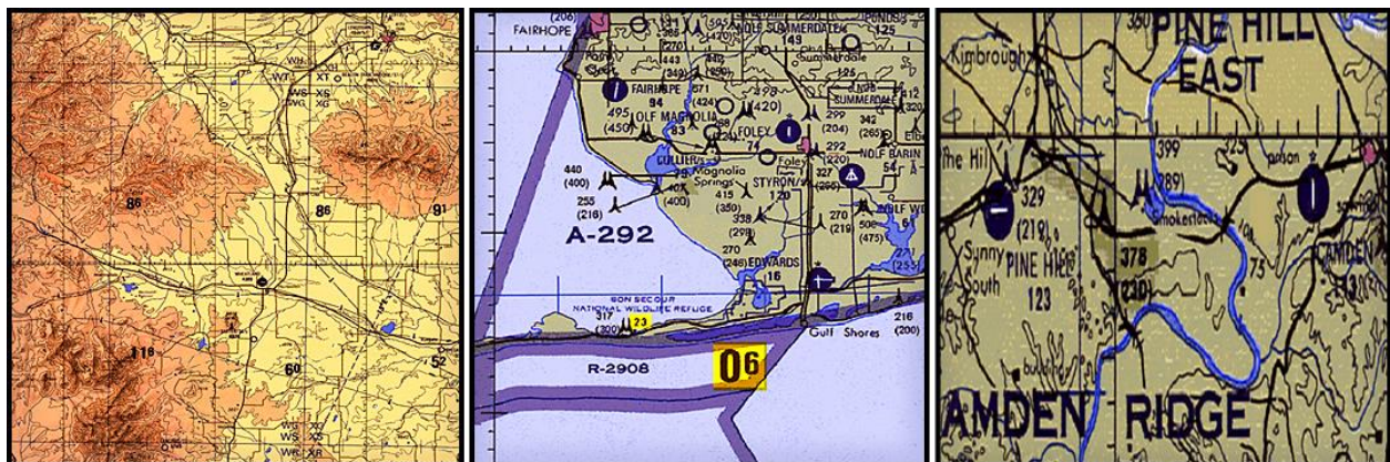
Figure 1-5 Contour Lines/Spot Elevations/Transportation Lines
