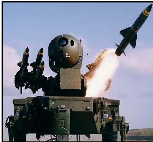
Figure 6-7 Combination Visual Tracking Ball on Rapier Surface to Air Missile System
