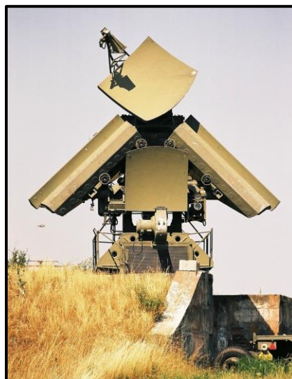
Figure 6-10 Low Blow Tracking Radar
