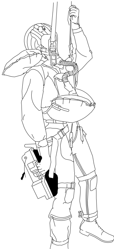
1. After inflating the LPU, prepare to deploy the seat kit.
