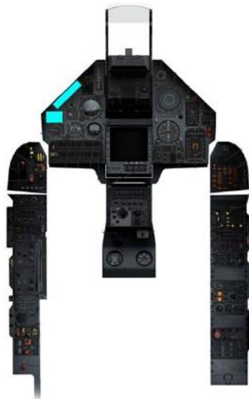
Figure 13 Autopilot panel location
