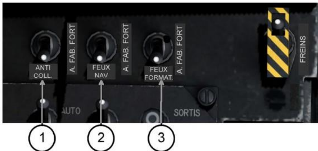
Figure 6 Exterior lights switches: Navigation, formation and anti-collision.
